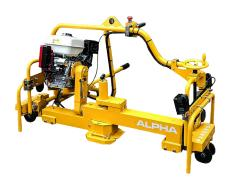
The Alpha Grinder extends the life of the track by grinding the complete profile in one operation, delivering the ergonomic design and precision efficiencies that Pandrol are renowned for.
